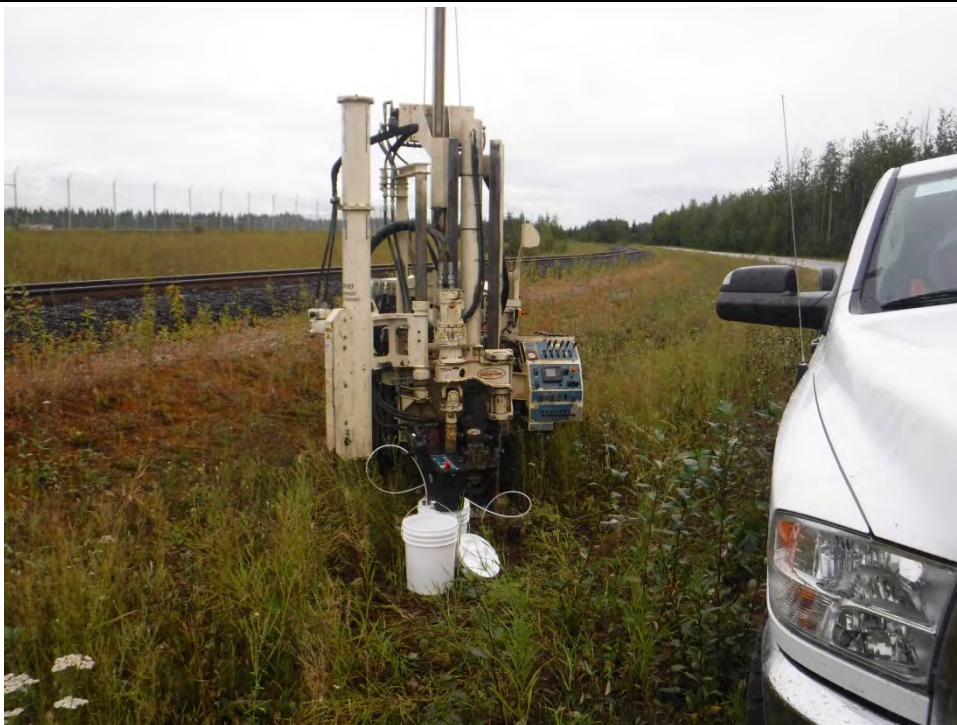
Description: Temporary monitoring well TW103a location and sampling set up.
